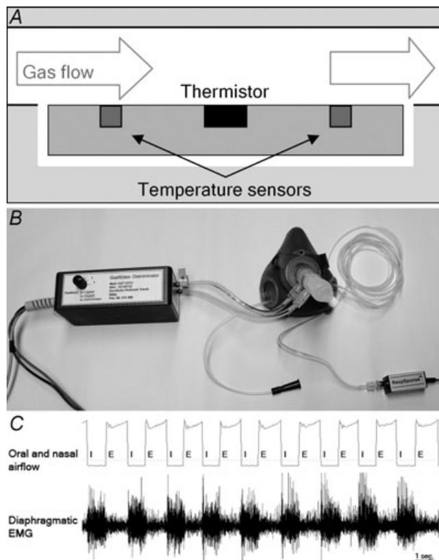
**Figure 1. The bidirectional gas flow discriminator**
